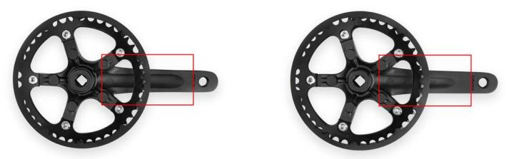
The indentation in the crank arm has a different appearance and there is also a raised dot to the left of the code on the replacement.
