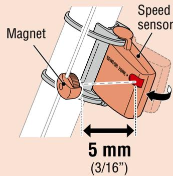
\* The magnet may be mounted at any position on spoke as long as attachment conditions are satisfied.
