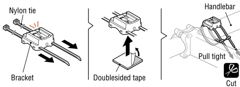
**When mounting the bracket on a handlebar, adjust the angle of the bracket so that the back of the computer faces the speed sensor when the computer is attached.**
